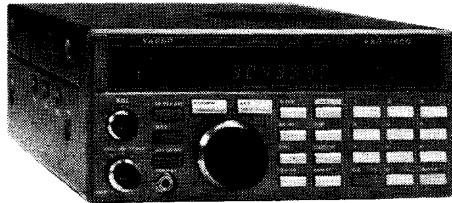
FT-757 GXII HF-TRANSCEIVER ALL MODE
